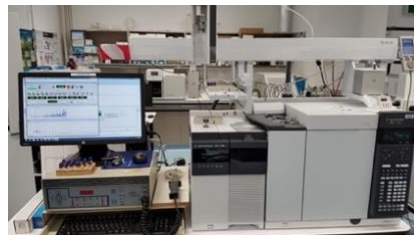
Photo. GCMS system used to characterise organic fractions during thermophilic composting
