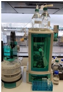
Photo. Ion chromatograph for measuring organic acids in fulvic acids
